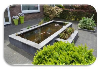
**VB-EPDM** prefab planters are available in almost any shape and size. They are easy to install in existing planters, but they can also be used as self-contained planters in green areas. VB-EPDM sheeting is resistant to root penetration in accordance with FLL guidelines. However, it cannot hold back some roots, for example the roots of certain bamboo and reed-like plants, for which alternative arrangements must be made.
